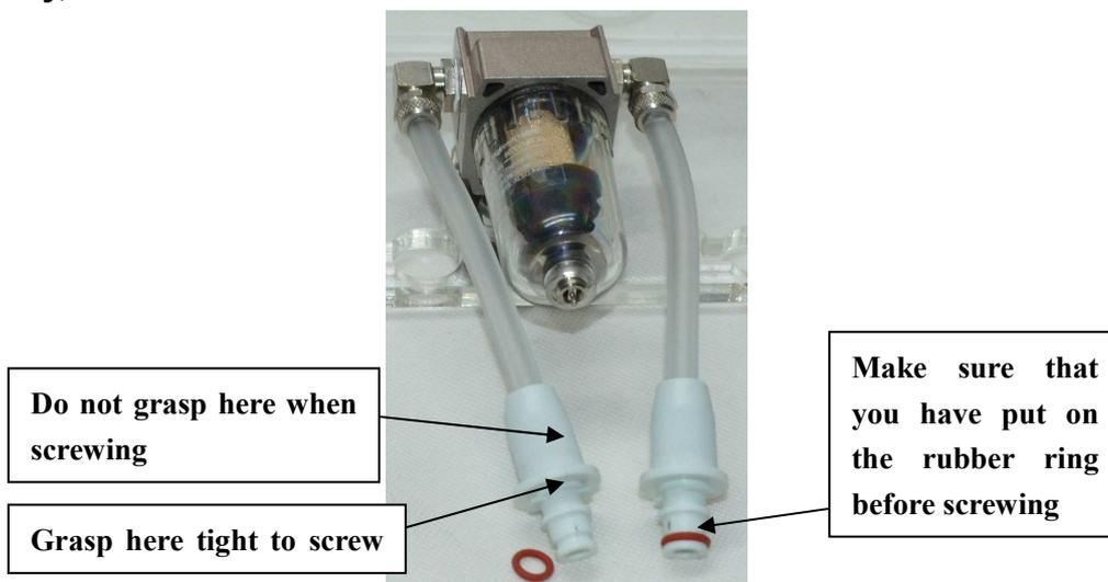
The filter should be clean every month. Take it off by contrarotation and clean with clear water. Make sure that you have screwed it up tightly after cleaning.
